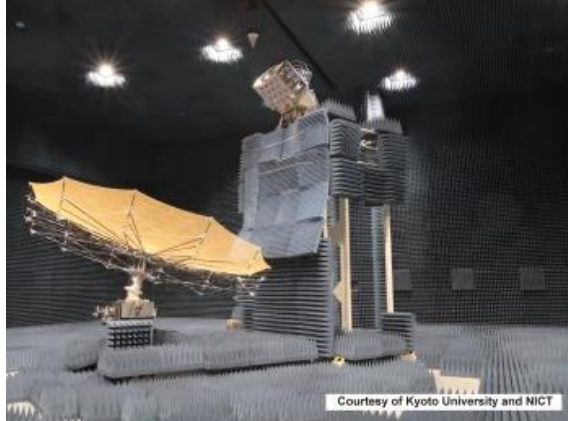
Figure 2. Kyoto University Plane Polar System with a 6 m Radius (12 m Diameter) Translation Axis
