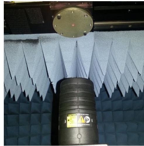
Figure 6. Axis Location Plate Mounted to Polarisation Rotator to Position Five Axis Laser Tool
