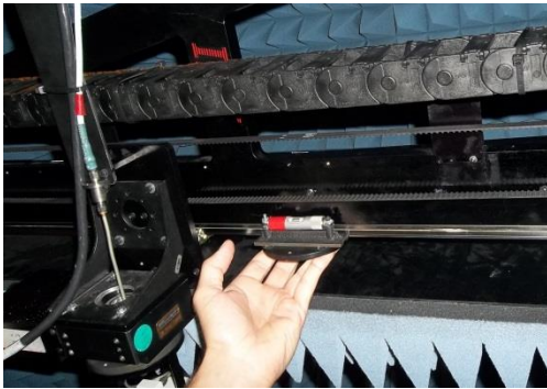
Figure 5. Checking the Radial Axis Level
