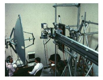
Figure 2 12' Diameter Plane-Polar System
