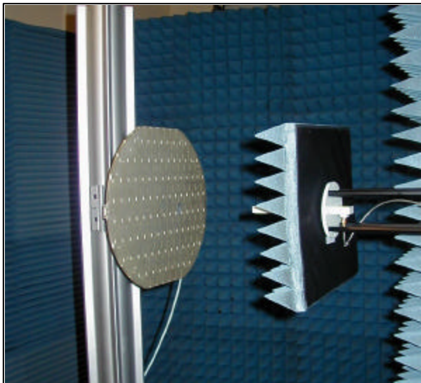
Figure 6 Slot Array test antenna in initial unrotated orientation.
