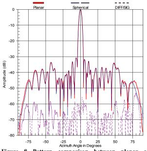
Figure 8 Pattern comparison between planar and spherical near-field measurements.
