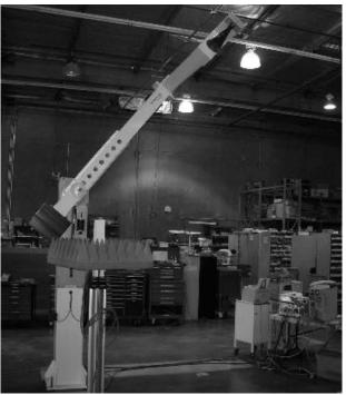
Figure 6 OEWG probe on the arch spherical range without absorber enclosure.
