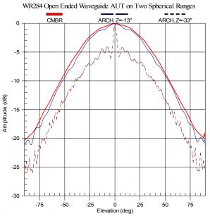
Figure 5 Far field patterns of an Open Ended Waveguide probe measured on three different spherical near-field ranges
