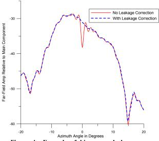
Figure 4 Example of bias error leakage on cross component data.
