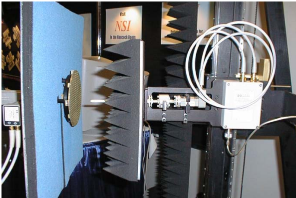
Fig. 7 Typical near-field probe mm-wave hardware and fixturing mounted on a planar near-field scanner.
