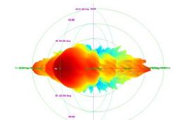
Fig. 11 Far-field pattern obtained from cylindrical measurement
