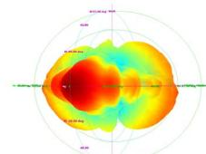
Fig. 10 Far-field pattern obtained from spherical measurement
