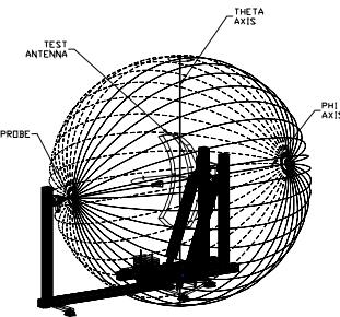
Fig. 1 Spherical positioning system and measurement geometry
