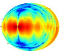
Fig. 3 Horizontally polarised measured spherical near-field component
