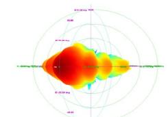
Fig. 13 Far-field pattern obtained from cylindrical measurement with cylindrical MARS processing
