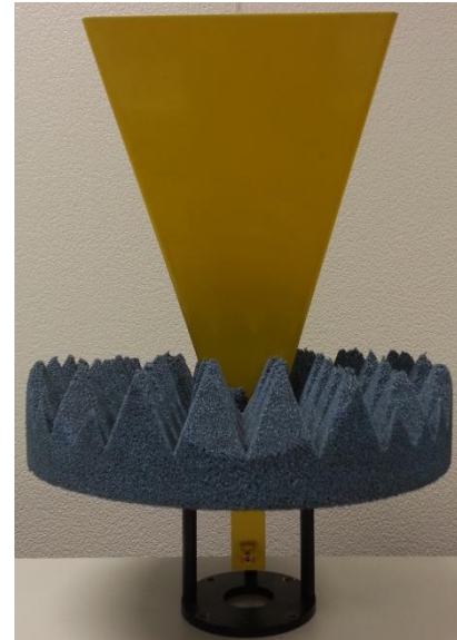
Figure 3. NSI-SG90 X-Band Standard Gain Horn Antenna used as Ant-2 in the Three-Antenna Gain Measurement and SGA in the Comparison Gain Method.
