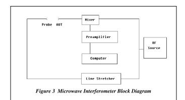
This design worked reasonably well for the intended application but suffered from several problems. The need for 2 measurement passes was not desirable and more importantly, this design was quite sensitive to mixer leakage and 1/f noise.
