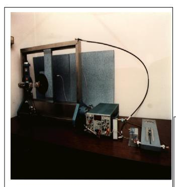
Figure 2 Near-Field Scanner withMicrowave Interferometer
