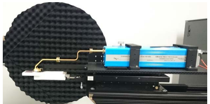
Figure 4. Low scattering, minimum blockage AUT probing system with millimeter head extension and waveguide connection
