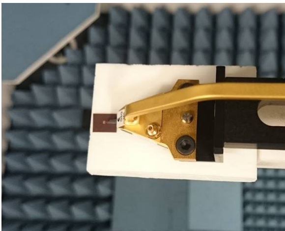
Figure 6. Patch antenna connected with a 250 \mu m RF probe
