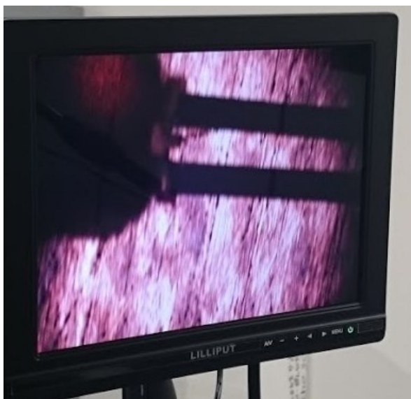
Fig. 3. Microscope view of the probing operation with a 250um GSG probe
