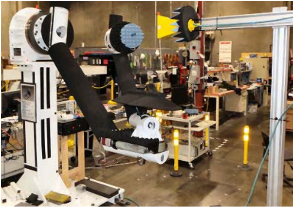
Fig. 2. Spherical near-field system undergoing factory testing. The stationary AUT can be seen positioned over the centre of rotation in a polar mode allowing near 4\pi steradian coverage with negligible blockage.
