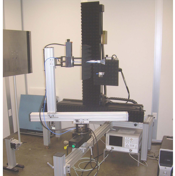
Fig. 3 NSI-200V-3x3 PCS system shown taking near-field measurements in a non-anechoic, office type, environment with a reflective plate shown to the left being used to increase range multipath effects.
