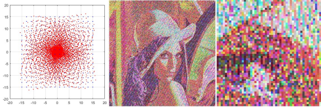
Figure 9. Constellation diagram and recovered image for the case of the massive MIMO antenna rotated to 30^\circ .
