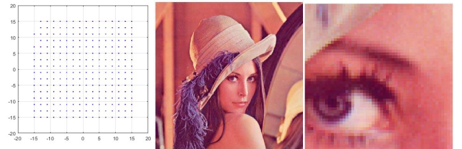
Figure 8. Constellation diagram and recovered image for the case of the massive MIMO antenna rotated to 10°.
