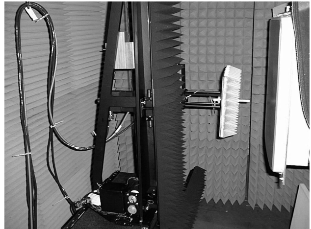
Figure 3: DVS antenna and nearfield scanner
