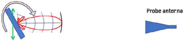
Fig. 10. Illustration of AUT rotated to 30^\circ with the beam electronically scanned back by 30^\circ to be directed towards the UE, i.e. probe antenna.
