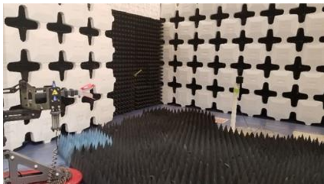
Fig. 2. Test setup showing EMC chamber with the remote source antenna seen to the left and the biconical to the right.
