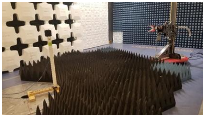
Fig. 3. Opposite view of test setup showing the offset biconical.
