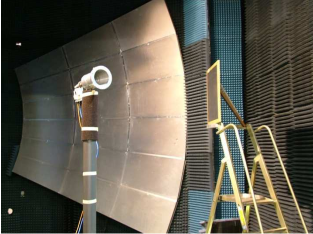
Fig. 1. X-band corrugated horn AUT installed within QMUL CATR shown together with 0.6 m X 0.6 m reflecting plate.
