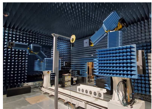
Fig. 1. Dual multi-axis industrial robotic antenna measurement system, picture courtesy of Boeing.
