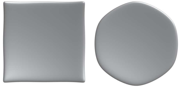
Fig. 9. m = 4 (left) and m = 6 (right) blended rolled edge reflector profiles.
