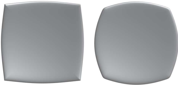
Fig. 2. BRE CATR reflector with standard JC (left) and equivalent SF based JC (right).
