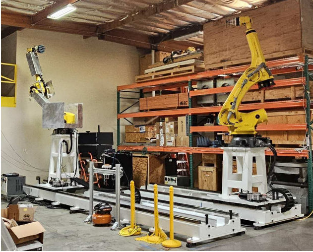
Fig. 1. Dual robotic antenna measurement system being used to acquire an x-band slotted waveguide array antenna in an open shop environment with no absorber and a large scatterer on one side of the acquisition.
